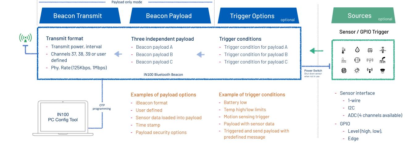
IN100 supports the latest Bluetooth 5 advertising extensions providing 255 bytes of message capacity and 40 channels of advertising capability, a boost from the 31 bytes and three advertising channels from the legacy BLE standard.
