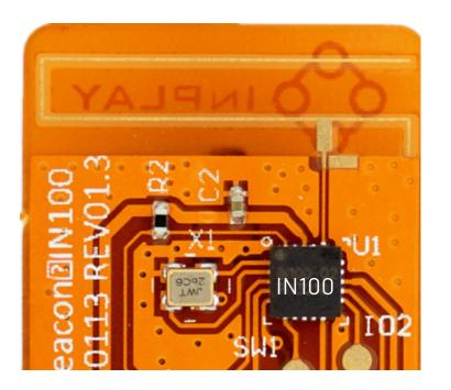
Average current of 1.4uA@ 10 seconds adv. interval Average current of 650nA@ 1 min adv. interval 500nA of sleep current
